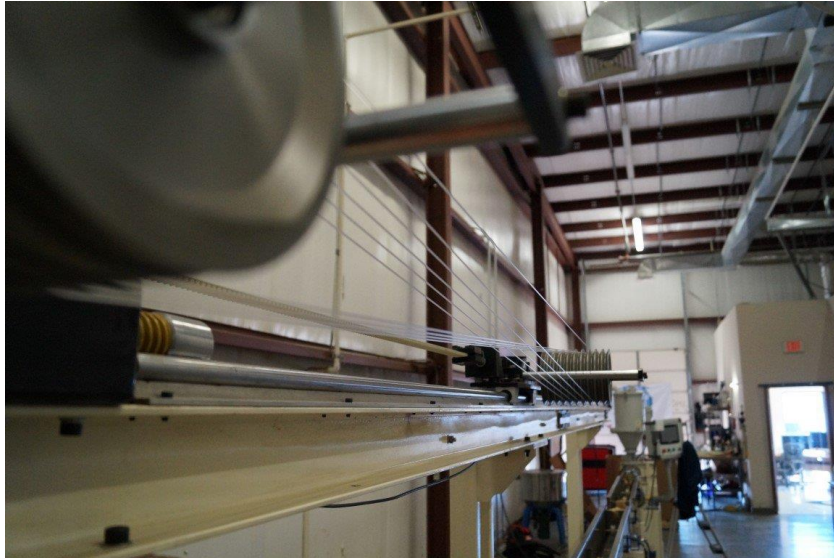
FIGURE 6 – Lines Of Filament Passing Through A Series Of Pulleys.
