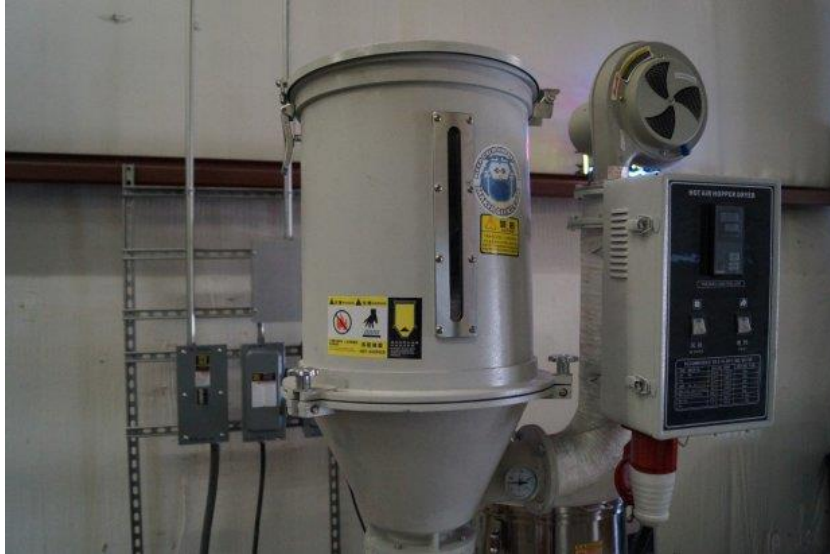
FIGURE 4 – Funneling & Hopper System
